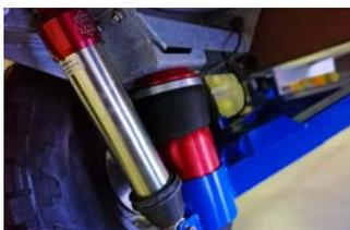
Monotube shocks & airbag suspension
