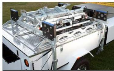
Boat Loader with Alloy Boat Trailer & Boat Risers
