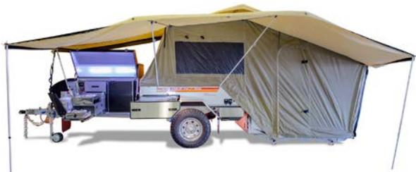
Kwik Awning with Vertical poles for wind & heavy rain conditions
